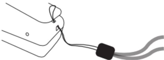
Step 1. Loop the thin end of the neck strap through the slot on the Headset.
