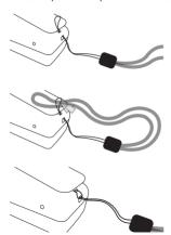
Step 1. Loop the thin end of the neck strap through the slot on the Headset.
